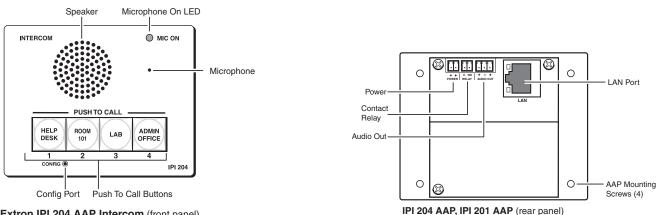
Extron IPI 204 AAP Intercom (front panel)
